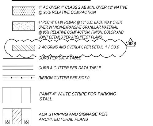
NOTE: THE PAVEMENT SECTIONS SHOWN ON THESE PLANS ARE FROM SOILS REPORT RECOMMENDATIONS. PAVEMENT SECTIONS WILL BE CONFIRMED ONCE SUBGRADE ELEVATIONS HAVE BEEN ATTAINED AND R-VALUE TESTING ON SUBGRADE SAMPLES IS PERFORMED.
